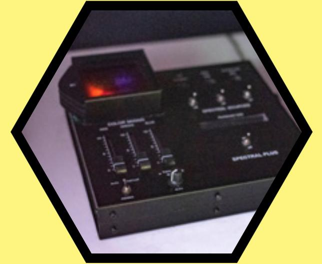
that the lights of the blue and green LEDs have “gone out”. This is because the red filter blocks all colours as we perceive them except for red. Try other colour filters in a similar way. There is also a multi-coloured plate, a CMYK filter. It consists of cyan (C), magenta (M) and yellow (Y). When these are mixed at the same ratio, black (K) is produced. Note that the basic RGB colours are obtained by mixing the following: magenta + yellow = red; yellow + cyan = green; cyan + magenta = blue.
