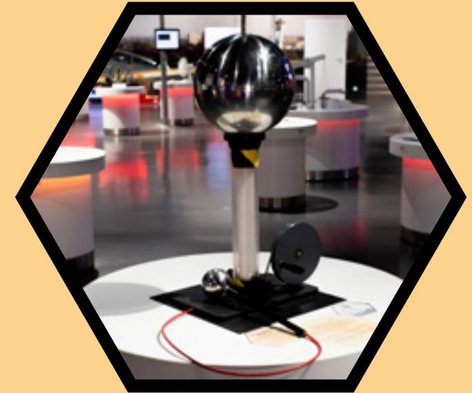
If you bring a grounded striker closer to a charged globe, you cause an electrostatic discharge.
