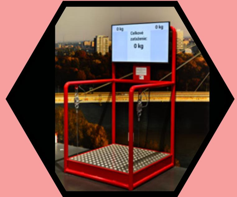
The functional model allows to test the location of the point load on the platform so that both ropes are equally loaded - achieving equilibrium. This is the principle of security, such as the statics of bridges or similar structures.
